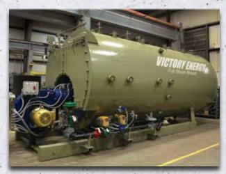
25,875 PPH - 750 HP - 150 PSIG - 3-pass packaged firetube boiler.
