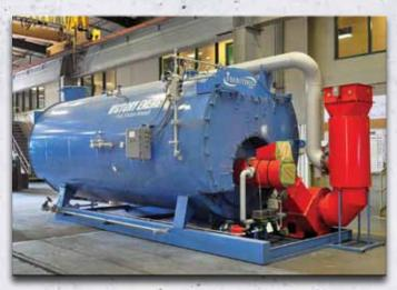
27,600 PPH - 800 HP - 300 PSIG - 3-pass packaged firetube boiler.
