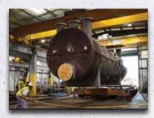
High pressure wasteheat sulphur recovery boiler.
