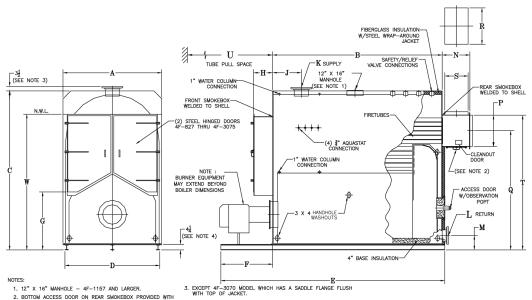
1. 12" X 16" MANHOLE - 4F-1157 AND LARGER 2. BOTTOM ACCESS DOOR ON REAR SMOKEBOX PROVIDED WITH REAR OUTLET ONLY.
