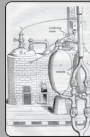
Thomas Savery patents “the Miner’s Friend,” a machine that pumps water from coal mines. It becomes the first practical machine powered by steam.
