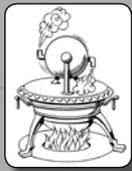
A Greek named Hero designed a simple machine (the aeolipile) that used steam as a power source to rotate a ball.
