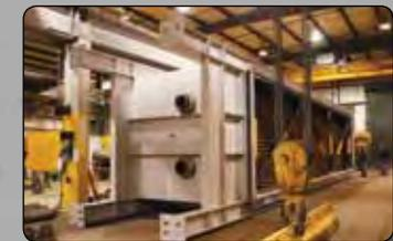
Final inspection of an HRSG module prior to shipment by rail.
