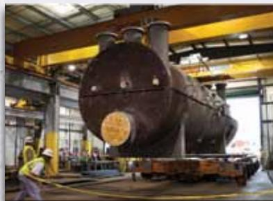
High pressure wasteheat sulphur recovery boiler.
